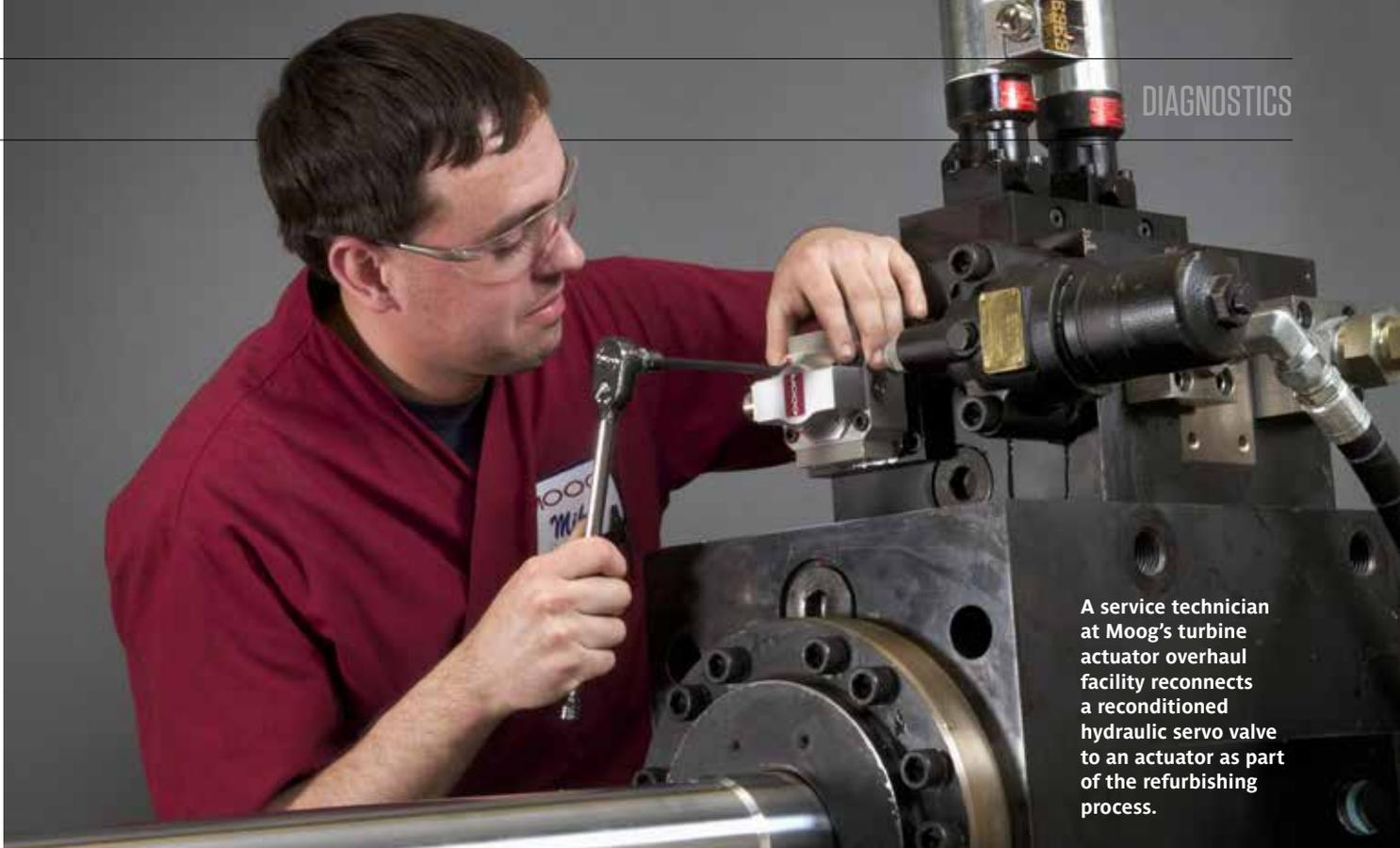
A service technician at Moog's turbine actuator overhaul facility reconnects a reconditioned hydraulic servo valve to an actuator as part of the refurbishing process.
