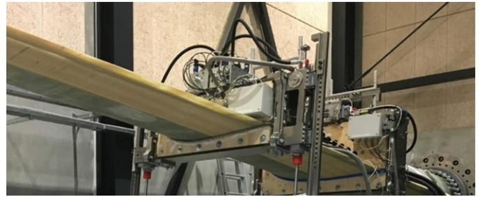
DTU researchers set up a blade test by attaching three hydraulically controlled MREs in DTU Large Scale Facility.
