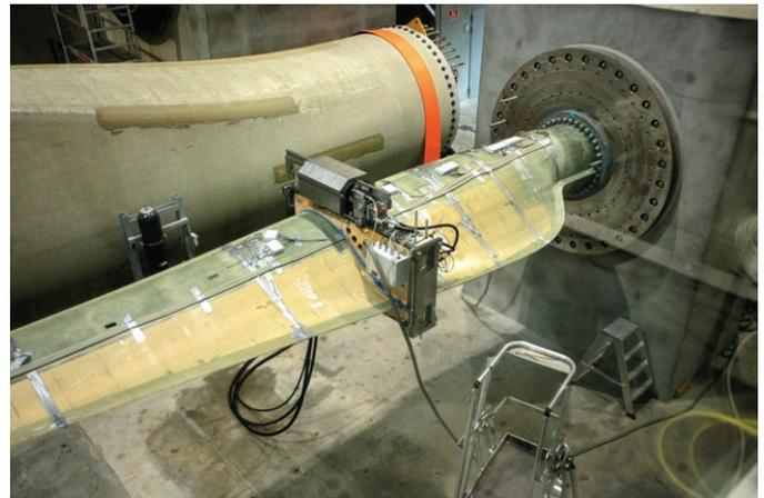
Mass resonance exciters (MRE), installed on a test blade at DTU Large Scale Facility.
